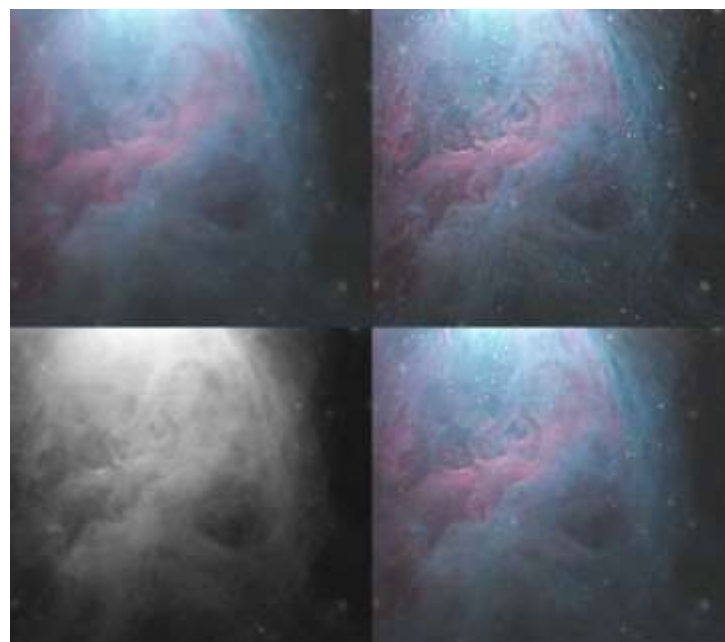
▲ Figure 2: TL: An image of the Orion Nebula. TR: The same image, after sharpening has been applied. Note the noise in the darker areas of the nebula along the bottom and right sides of the image. BL: A mask made from the original nebula image. BR: The sharpened image, with the mask applied to the sharpening function. The darker areas appear smooth. See the full sized image at http://tinyurl.com/zll5d7x (Photo: Art Cole).
