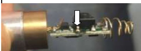
Tristan discovers poor soldering on laser circuit board. (Photo: Tony Schellinck)
