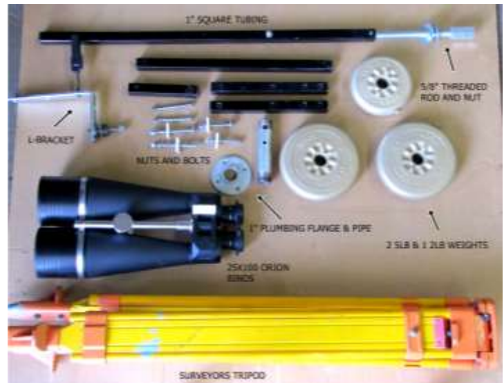
Parallel Mount Components (Photo: Wayne Mansfield).
