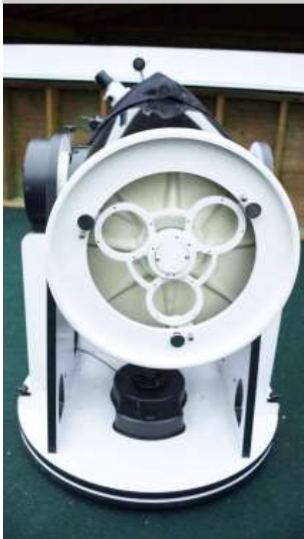
Collimation knobs at the base of the Sky-Watcher SynScan altazimuth Dobsonian telescope. (Photo: Halley Davies)
