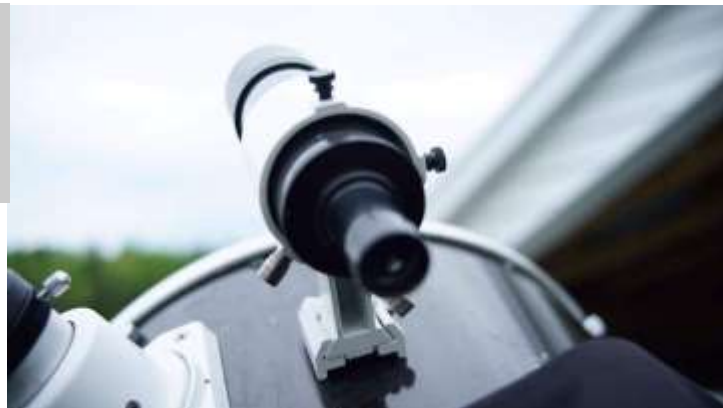
The 8x50 inverted-image optical finder with crosshairs on the Sky-Watcher Dobsonian telescope. (Photo: Halley Davies)
