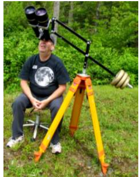
Wayne tests out his DIY parallel binocular mount (Photo: Pam Mansfield).
