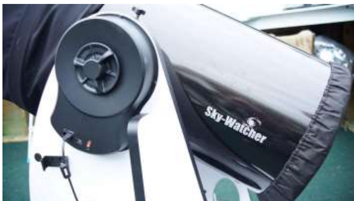
The hand clutches on the side and base are loosened when pushing the scope by hand and tightened when using the hand control to reposition the telescope. (Photo: Halley Davies)
