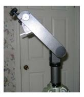
CAUTION – Caution must be exercised when using the binoculars with the mount in the 45 degree orientation. In this configuration, the centre of gravity of the binoculars is behind the vertical axis of the tripod. While this is a reasonably stable configuration, if the binoculars are bumped with sufficient force, they could be knocked over.
