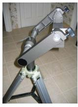
The amount of effort required to move the binoculars in altitude is adjusted by tightening the two knurled knobs overtop the swing bracket bearings. This is a finger tip adjustment. Avoid over tightening. Always store the binoculars with the pressure on these bearings released.
