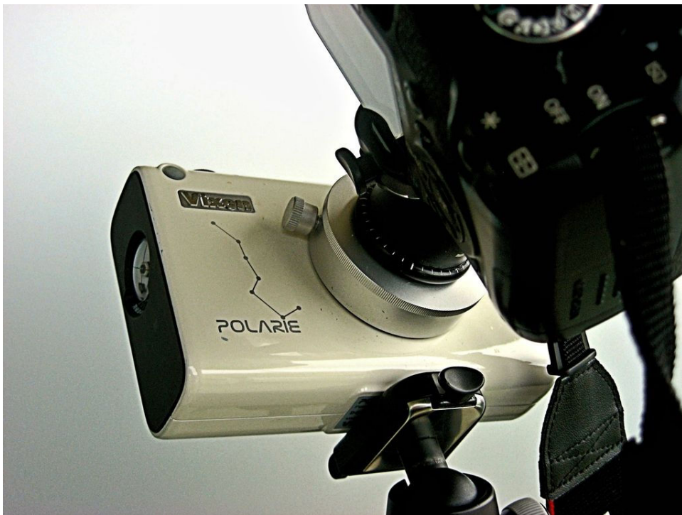
Photo: John McPhee Close up view of the Vixen Polarie camera tracker mounted on a ball end tripod, with a camera mounted on the output shaft.
