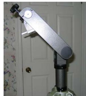
**CAUTION** – Caution must be exercised when using the binoculars with the mount in the 45 degree orientation. In this configuration, the centre of gravity of the binoculars is behind the vertical axis of the tripod. While this is a reasonably stable configuration, if the binoculars are bumped with sufficient force, they could be knocked over.
