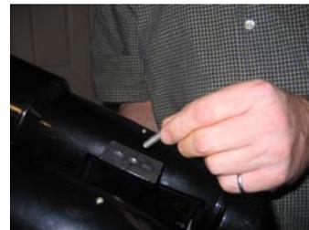
Still holding the binoculars by the handle, insert the threaded rod into the hole in the swing bracket as indicated in the photograph at right. While holding the binoculars in place with one hand, centre the binoculars on the swing bracket so that they sit square with the mount. Secure the binoculars to the swing bracket using the attachment bolt. Do not let go of the binoculars until you have tightened the knob securely.
