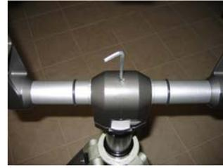
While holding the fork with one hand, slowly loosen the set screw until the fork moves easily. Notice that the circular shaft which passes through the top of the pillar has index marks on the raised section of the shaft inboard of the two black O-rings. These detents indicate the 45 degree setting of the fork.
