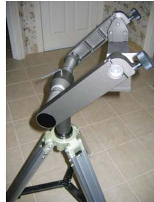
Once the set screw is loosened position the forks such that the 45 degree detent is under the set screw. Ensure that the shaft remains centered by observing that the black O-rings remain equidistant from each edge of the pillar. Slowly tighten the allen key while ensuring that the detent remains properly positioned underneath the set screw. Continue to tighten the set screw until secure. Remove the set screw and replace the back plug.
