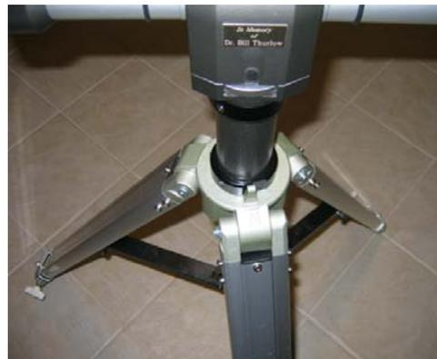
The amount of effort required to move the fork in the azimuth is controlled by a knurled ring which is partially exposed on the front face of the mount just above the pillar.
