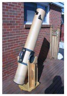
The hinged plywood box was replaced with a much lighter design with cut back the amount of wood that was used. Mike was very pleased with the results. The original scope was 31 lbs and the rebuilt one was only 23 lbs, a saving of 8 lbs. Mike utilizes this excellent handmade scope to produce really great sketches of the planets, that and can be seen on the Halifax center website.
