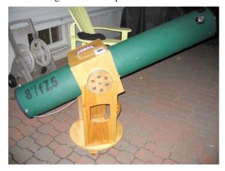
This scope was made of 2 Sonotubes placed one inside the other. The inside was flocked and the outside was covered with a plastic coating. A hinged plywood box held the scope and the altitude bearings. The scope worked well for Mike but was heavy and after years of faithful duty began to show the effects of much use.
