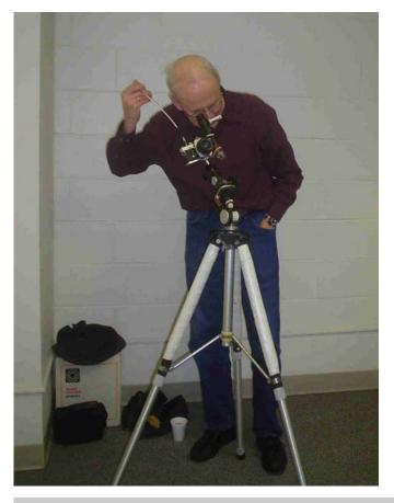
The mount is actually a small piggyback mount that has dual axis motion and has slow motion controls. This mounts on the camera tripod. Using a small wooden triangular jig, Roy adjusts the angle of the mount for the latitude he is observing at. Once the correct latitude was set Roy showed how he would sight along the side of the mount to line everything up with Polaris. With the mount all lined up his camera is attached to a ball mount, which allows the camera to move in all directions.
