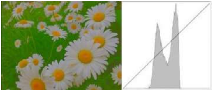
▲ Figure 2: A low-contrast version of the image. The histogram shows how the pixel intensities are constrained to a narrow band. (Photo: Art Cole).
